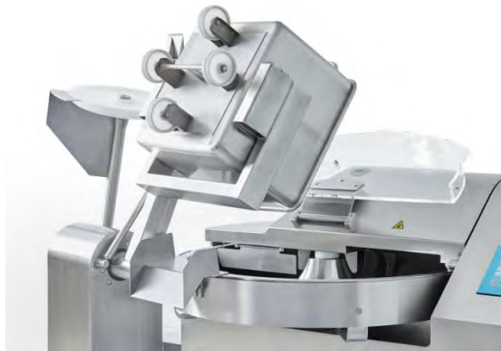
Hydraulic loader for fast and simple filling. Standard 200 l trolleys.
