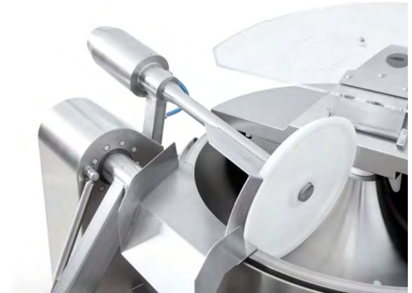
Hydraulic and motorized unloader for emptying the bowl fast and simple.
