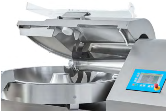
Stainless steel motorized knife lid for effortless lifting and lowering.
