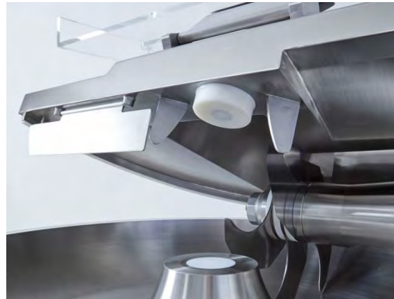
Smooth polished surfaces , no corners or screws, with C\infty radius for easy cleaning.
