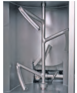
Stainless Steel Feedscrew and Mixing Paddle
